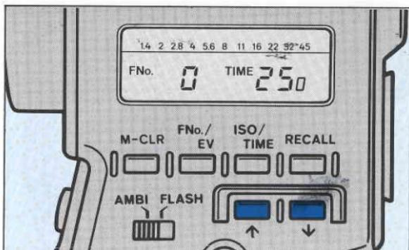
To change the shutter speed, press the increase or decrease key until the desired speed is displayed. Each time either key is pressed, the display will change by one full stop. The speed changes continuously when either key is held down.
