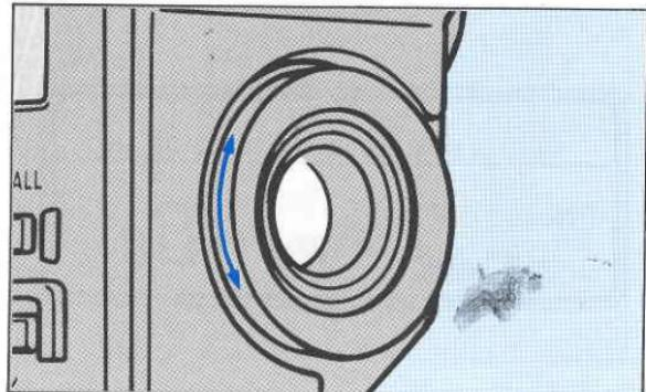
The Spotmeter F has a fixed-focus objective lens that provides correct focus from 1.3 meters to infinity.
