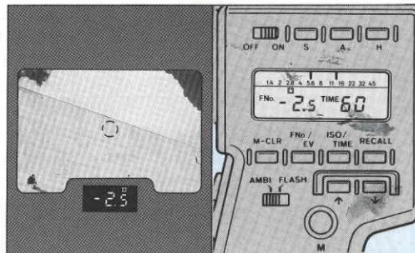
A mid-tone reading was used for this example, however, similar readouts appear for highlight, shadow and averaged readings.
