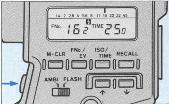
5. Press the measuring button to fire the flash and take a reading.
