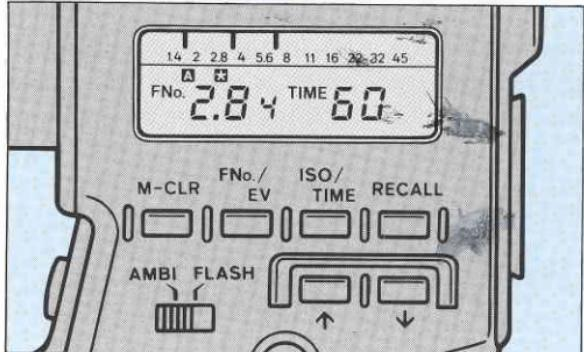
digital readout. This second reading can be entered by pressing the memory key again.
