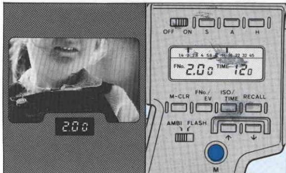
When the averaging key is pressed, **A** and **■** will appear on the digital display along with the calculated exposure. A third pointer will appear on the analog scale between those of the memorized readings.
