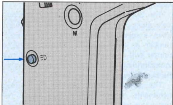
The viewfinder display can be illuminated for easier reading in low light by pressing the display illumination button located on the meter's grip.
