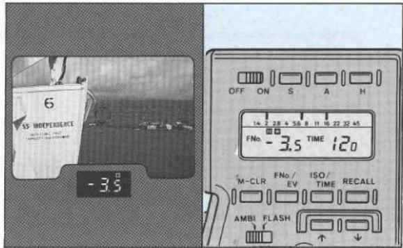
If another reading is made when the **\*** mark is displayed, the meter will indicate the difference in brightness between the calculated reading and the new reading. Refer to page 36 ~ 38 for more information.
