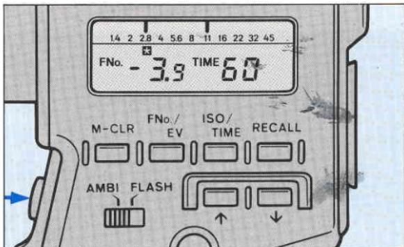
For example, after taking a reading of a highlight area and pressing the "A" key, you can take readings of various shadows to check the difference in brightness of these areas. As the readout above indicates, the shadow area is 3.9 stops darker than the highlight area.
