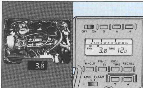
If another reading is made when the  $\oplus$  mark is displayed, the meter will indicate the difference in brightness between the calculated reading and the new reading. Refer to page 36 ~ 38 for more information.
