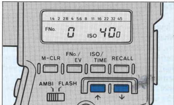
2. Press the increase key to set higher film speeds; press the decrease key to set lower film speeds. The setting changes by 1/3 stop each time either key is pressed and continuously when a key is held down. Any film speed from ISO 12 to ISO 6400 can be set.
