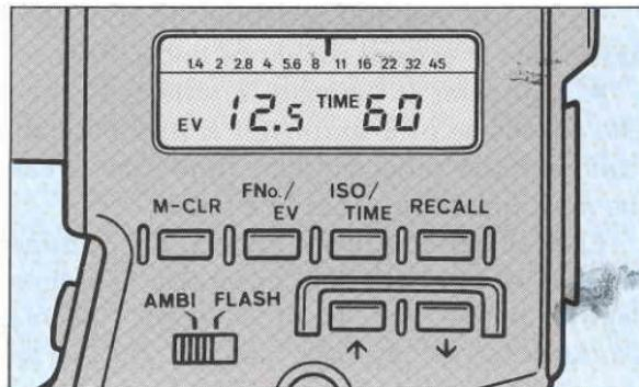
The EV display mode is useful for checking contrast ratios (p. 39), luminance (p. 40), and other lighting conditions. In this mode, the display readout will be in EV steps, and only changes in the ISO setting will affect the EV display.
