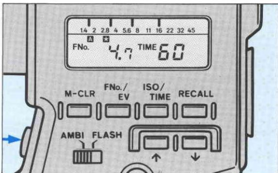
on the analog scale next to indicated the f-number. A  $\pm$  mark will also appear indicating that any further readings will be displayed as differences in brightness from the calculated reading. These readings will also be indicated by a fourth pointer on the analog scale. Refer to page 36 ~ 38 for more information.
