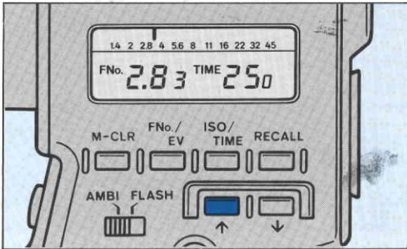
If desired, other aperture/shutter speed combinations can be displayed by pressing the increase or decrease keys.
