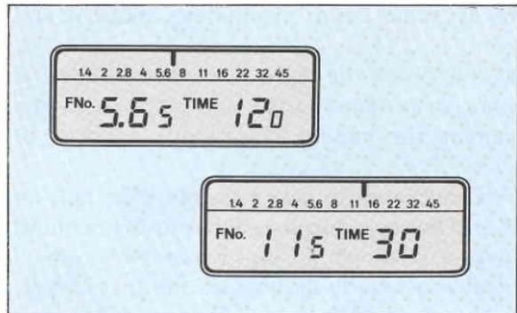
When taking ambient-light readings, changing the ISO or shutter-speed setting will change the f-number displayed.
