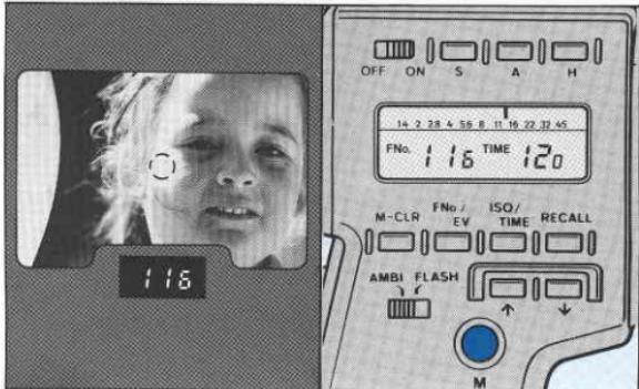
To obtain an average exposure for a scene, first measure a bright highlight and press the memory key to enter the reading into the meter's memory. Then measure a dark shadow and memorize this reading. Now, press the averaging key to calculate the average exposure.
