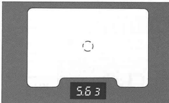
In addition to the meter's external display, there is also a digital display in the viewfinder that lets you monitor the exposure information while taking a reading. The f-number, EV number, and brightness differences are displayed with tenth-stop accuracy. The measuring spot defines the meter's  $1^{\circ}$  angle of acceptance.
