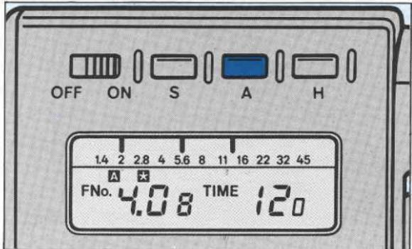
If another reading is made when the **\*** mark is displayed, the meter will indicate the difference in brightness between the averaged reading and the new reading. Refer to page 36 ~ 38 for more information.
