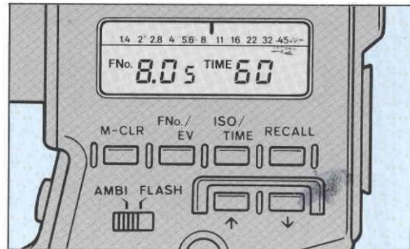
The Spotmeter F has two display/measurement modes, f-number (FNo.) and exposure value (EV). Press the FNo./EV key to display the desired mode on the external LCD display panel.
