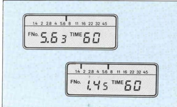
To use the Spotmeter F's memory function, take a reading and press the memory key. The display will go blank for a moment and then reappear after the reading is entered into the memory. You can now take a second reading which will be indicated by a pointer on the analog scale and by a new
