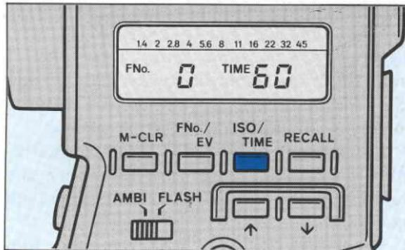
After setting the film speed, press the ISO/TIME key to put the meter in time-display mode. The display will show the most recently set shutter speed. If the battery has just been installed, "60" (1/60 sec.) will be displayed.
