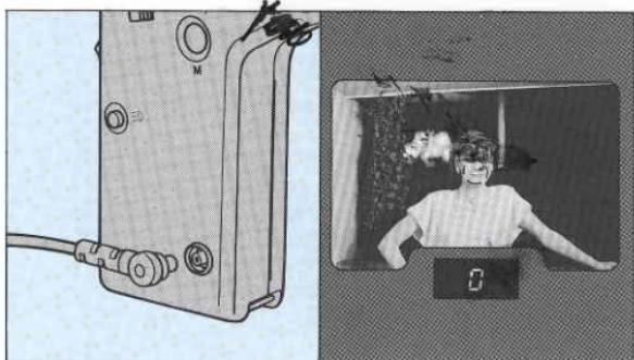
1. Set the metering-mode switch to "FLASH". F-number display mode will be set automatically.
