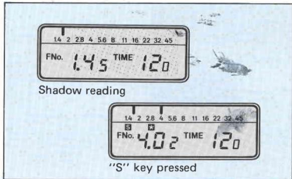
To make a shadow reading, first press the memory-clear key to clear any previously memorized readings, then proceed as follows:
