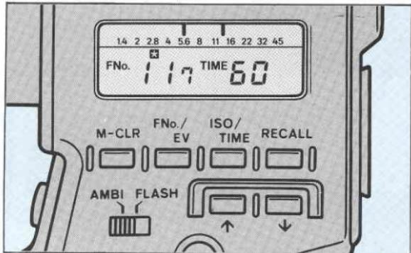
4. When you release the measuring button, the calculated exposure will be displayed again.
