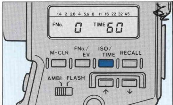
3. After setting the film speed, press the ISO/TIME key to return to the time-display mode.
