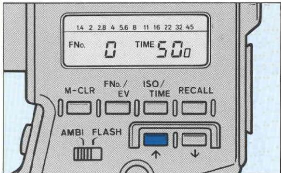
In ambient metering mode, the shutter speed can be set from 1/8000 sec. to 30 minutes, plus 1/50 sec. (which comes after the 30 min. when pressing the decrease key) for taking cine readings at 24 fps.
