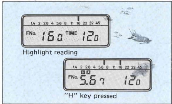
To make a highlight reading, first press the memory-clear key to clear any previously memorized readings, then proceed as follows:
