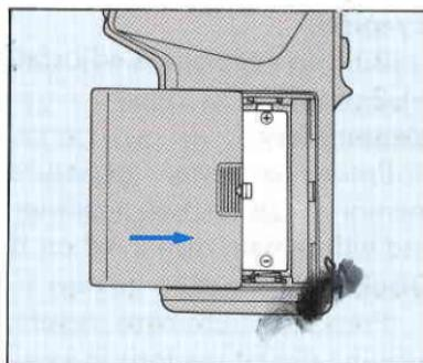
The Spotmeter F is powered by a single AA-size battery. A 1.5-volt alkaline-manganese or carbon-zinc battery or 1.2-volt nickel-cadmium battery can be used. To install the battery:
