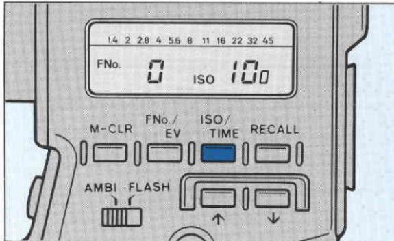
1. Press the ISO/TIME key to display the ISO film-speed setting. If the battery has just been installed, "100" (ISO 100) will be displayed.
